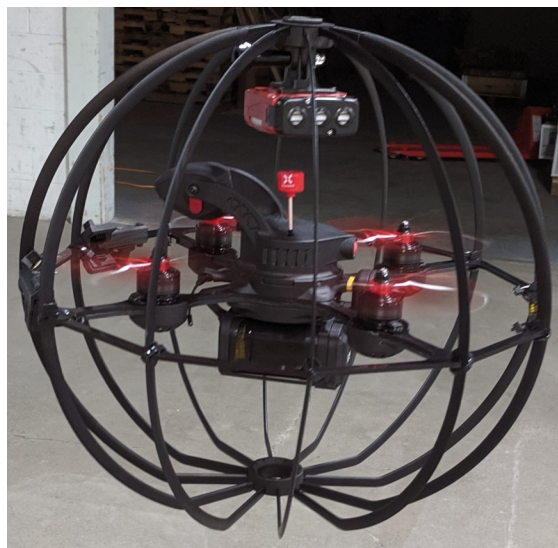
SkyCopter 2.0 Cobra equipped with Gas Detector
