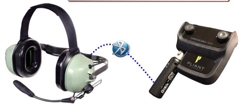
The Wireless HBT- 40 connects via Bluetooth 4.0 to the BlueNet adapter connected to a CrewCom Radio Pack.
