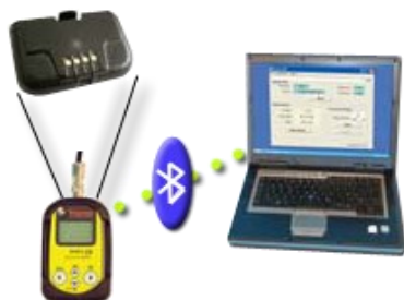
RadEye BTcom cover for Bluetooth® communication
