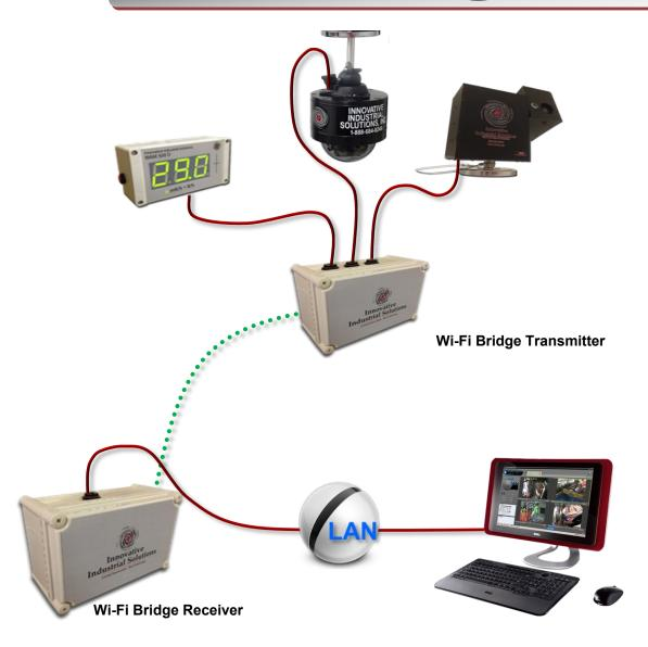
The I.I.S. Wireless Bridge Receiver will connect up to 3 I.I.S. Wireless Bridge Transmitters which has 3 PoE Ports and will connect up to 3 cameras each or 2 cameras and one PoE device (WAM or Power over Ethernet Light)
