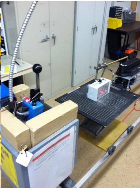
Figure 4 – Unit Rotated 270 Degrees (beam directed to right side of monitor)
